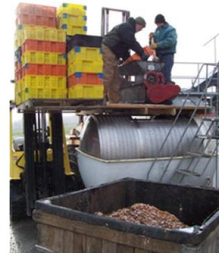
During pressing, a thick concentrated juice trickles out of the press and is pumped into a stainless steel tank. After an entire load is pressed, the frozen residue has to be chiseled out of the press. This residue is composted and spread back in the vineyards as fertilizer.
