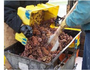
The frozen grapes are forced into a crusher. The crushed grapes fall through a hole in the platform into our special basket press (below, steel-colored).
